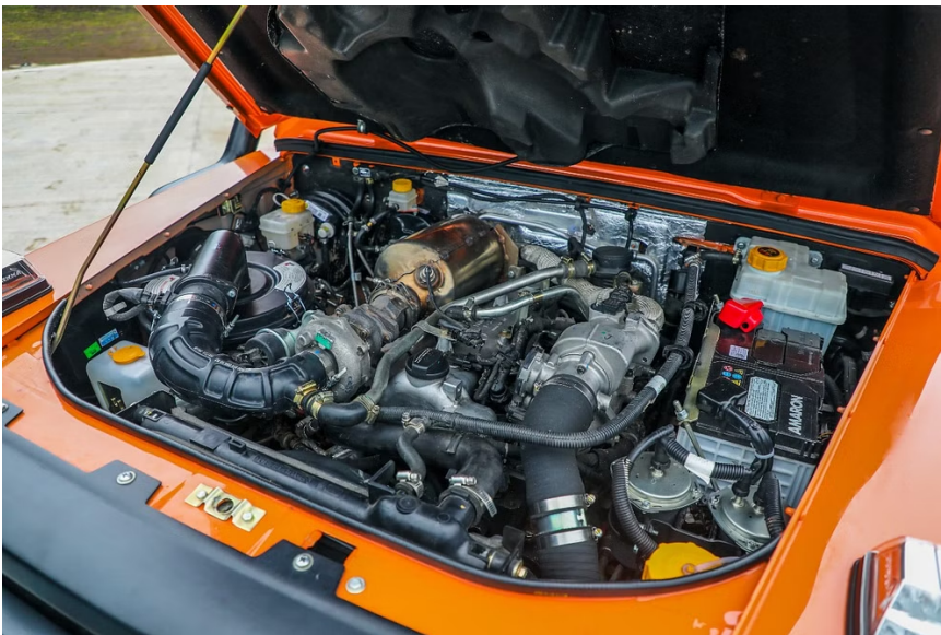
The 2021 Gurkha gets the OM 616-derived 2.6-litre diesel engine that produces 88.7bhp and 250Nm Team evo India
